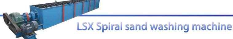
Trough: It contains shell, input devices, right weir plates and left weir plates. Trough is steel plate jointed into water tight structure. Right and left weir plates and input devices are connected by bolt, nut, and grower washers. Right weir plate and left weir plate &=3(mm)rubber sheet for sealing.
