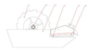
1.bucket (single, double or triple)2.LYC bearing 3.water tank4.rubber spring 5.motor6.PU screen (thickness 45mm)
